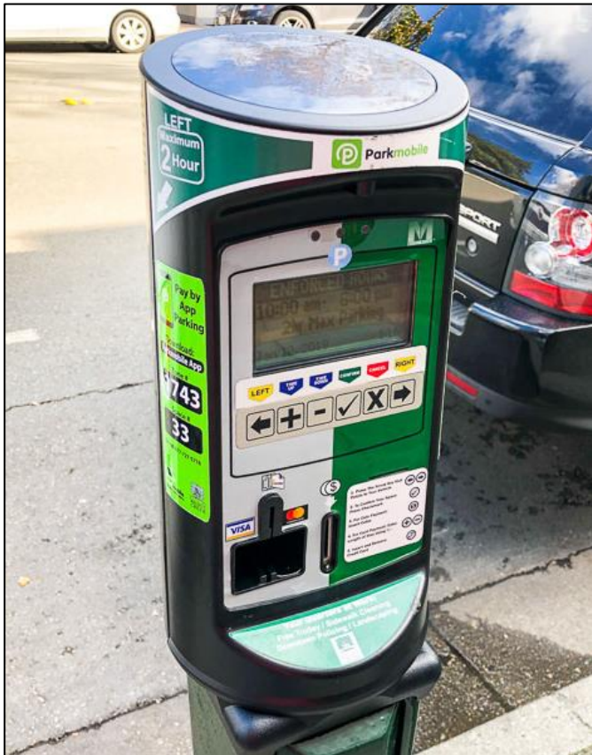
Figure 1: Dual-Space Smart Parking Meter in Walnut Creek
