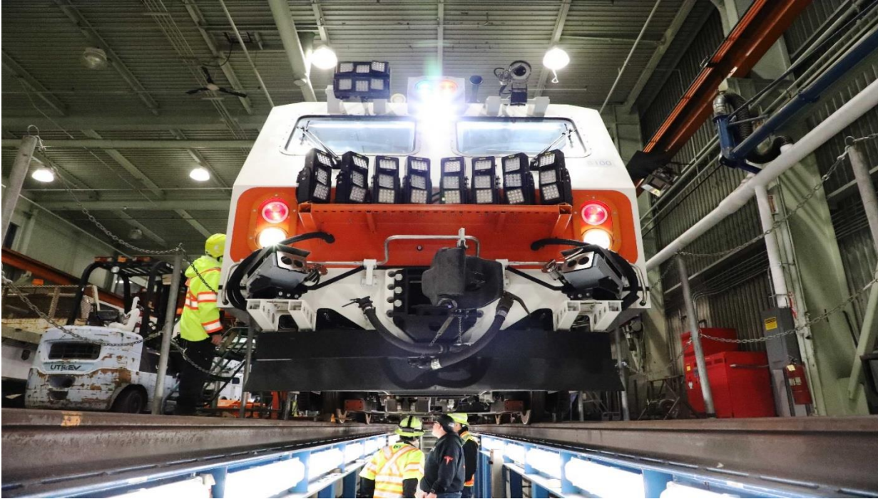
Description: Geometry Car preparing for rail inspections and maintenance.
