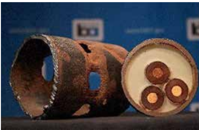
Decayed old cable, left, and modern insulated cable, right
