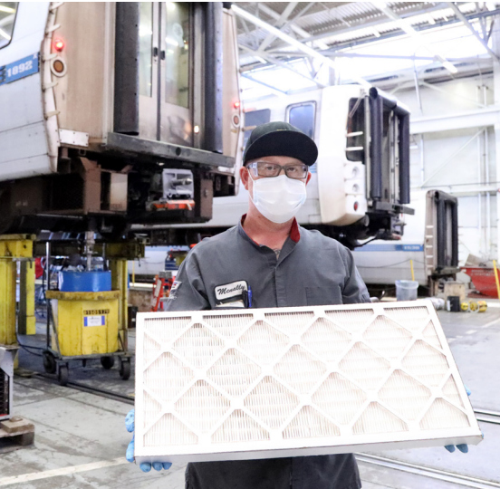
The ventilation systems installed on the BART fleet replaces each car's air about every 70 seconds.
